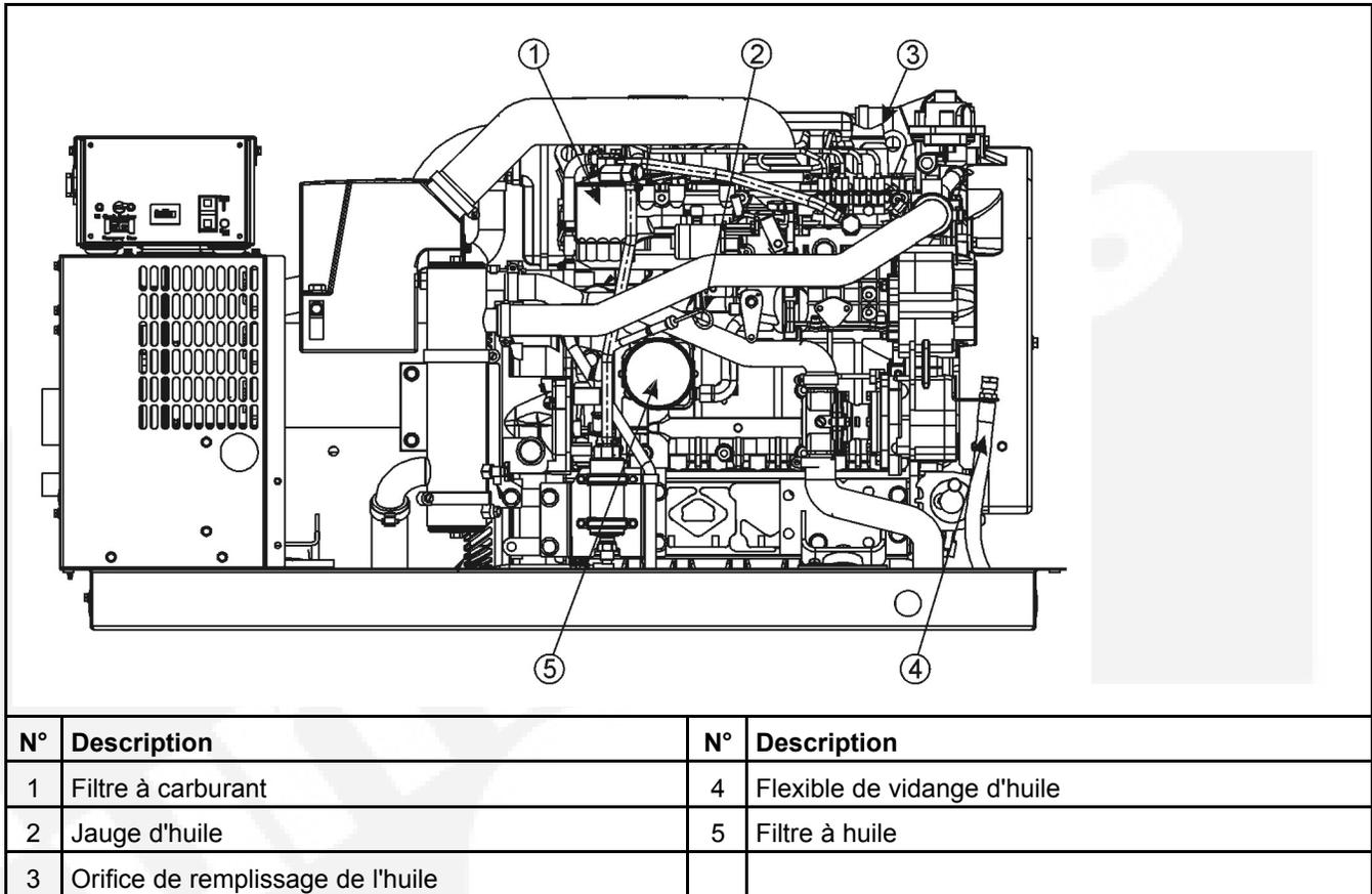
FIGURE 14. POINTS D'ENTRETIEN DE L'HUILE ET DU CARBURANT - MDKDS, MDKDT, MDKDU
