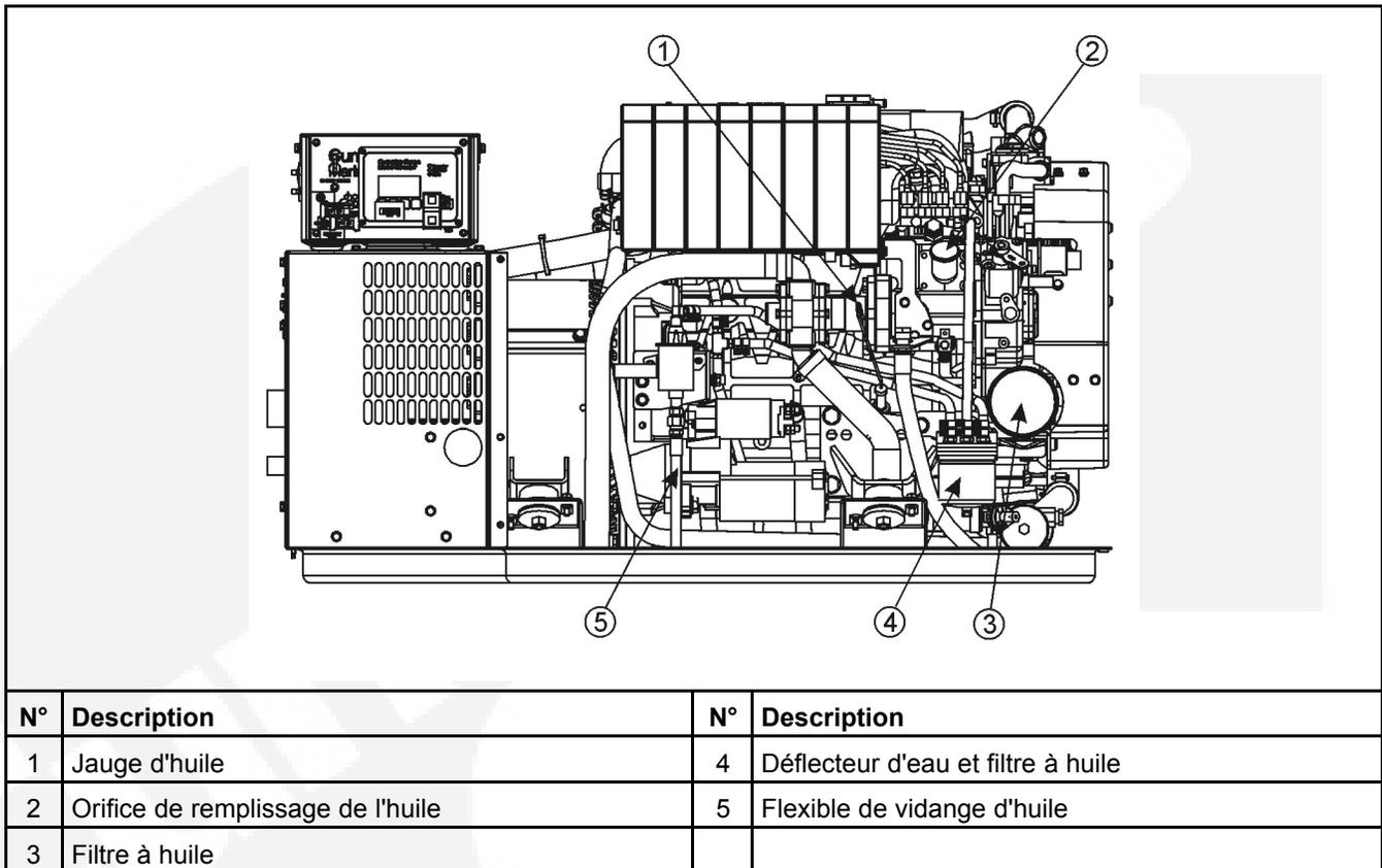
FIGURE 13. POINTS D'ENTRETIEN DE L'HUILE ET DU CARBURANT - MDKDP, MDKBR, MDKDV
